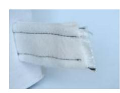
OUTER LAYER – spun polyester geotextile covering the core 1.5 times.
