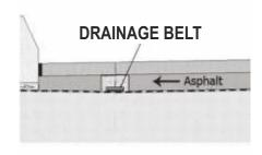
A slight elevation difference from end to end is all that is required to activate drainage on horizontal surfaces or uphill slopes.
