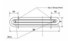
**DB** may be laid underneath or inside drainage systems and between steel or concrete structural members and asphalt.
